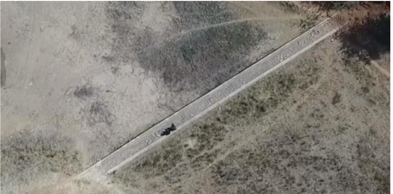
Figure 20: Service spillway showing need for abutment protection
